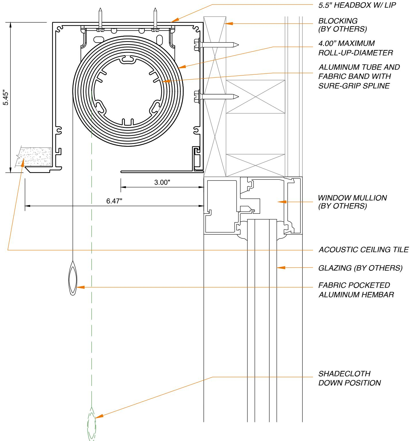
\*NOTE: POCKET SHOWN AS WALL MOUNT, CAN ALSO BE CEILING MOUNT, OR INSIDE FRONT MOUNT IF PROPER BLOCKING IS PROVIDED
